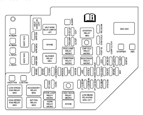
The underhood fuse block is located in the front of the engine compartment on the passenger's side of the vehicle. See *Engine Compartment Overview on page 373* for more information on location and removal procedure for the front compartment underhood sights shields.
